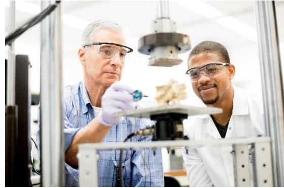
Jeffrey Lotz, PhD, left, and graduate student Devante Horne examine vertebra using a material testing system
