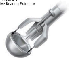
Figure 48 Placement of Alternative Bearing Extractor
