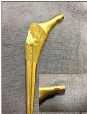
Figure 2: Postoperative photograph of the retrieved stem from Patient 1, showing severe trunnion wear and deformation. The inset illustrates the femoral head notching of the trunnion.
