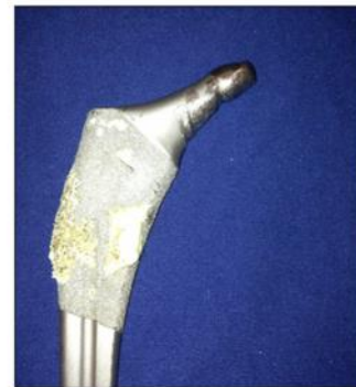
Figure 4: Postoperative photograph of the retrieved stem obtained from Patient 2, showing similar trunnion wear and deformation as seen in Patient 1, with deep grooves in the inferior femoral neck.
