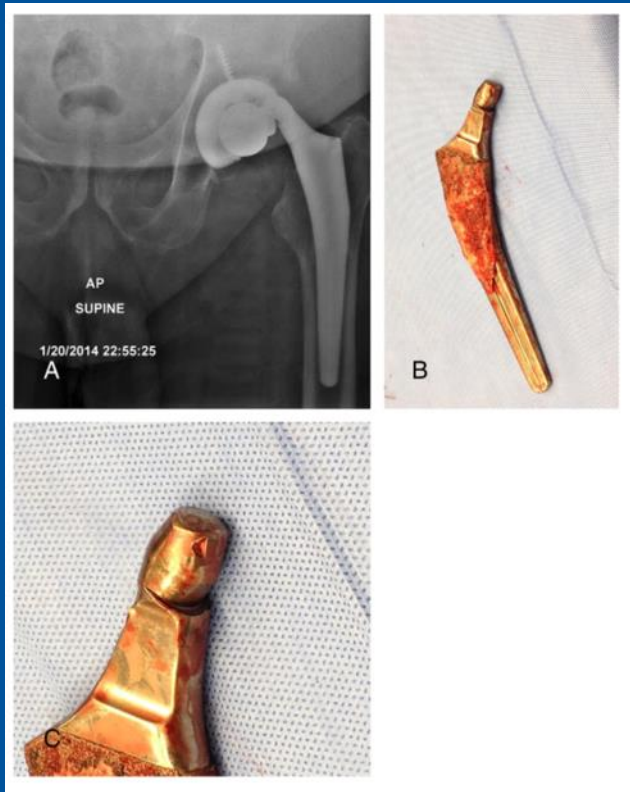
Fig. 2. (A) and (B) Initial radiographic images on presentation (patient 2) showing dissociation of the trunnion from the femoral head.
